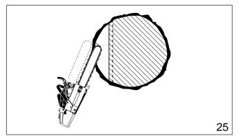
in which the recess is to be cut. With the saw at full throttle, insert the guide bar in the trunk (fig. 27).
